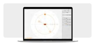
Symphonia's advanced algorithm reproduces background noises recorded with special multichannel microphones, to make the patient feel inside a realistic external environment. Voices or musical instruments can be added to the sound field and moved all around the patient, to simulate directional sounds coming from different directions.
