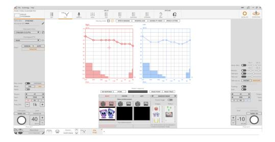
This system enables precise pure tone audiometry while providing seamless control over the reinforcement stimuli. The reinforcements, which include LCD displays showing engaging images or animated toys, are directly integrated with the device. Additionally, the use of the assistant monitor, which can be activated via software, significantly enhances the overall efficiency and accuracy of the testing process.
